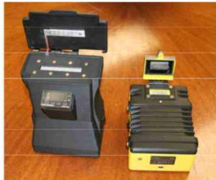
Figure 1. Two version of the Rabbit Fluorimeter. Version 5.2 (left) and version 6.1 (right). On board display and controls are available.
