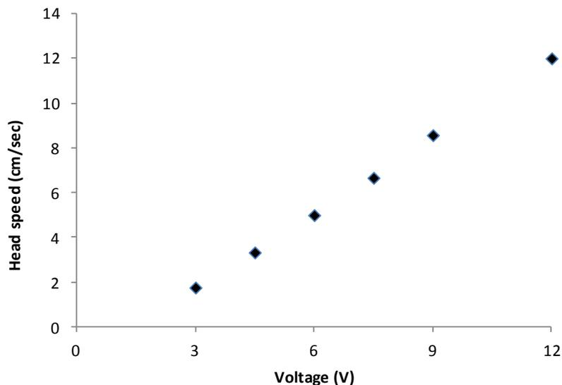
**Figure 1 Voltage dependence on head speed:** Voltage of LFRD varied from 3 - 12v. Distance travelled = 30 cm.
