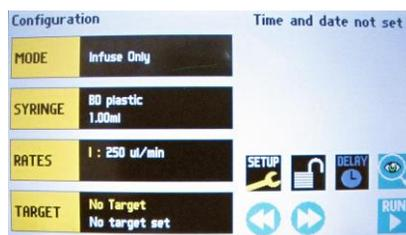
**Figure 4.** Syringe pump configuration touch screen
