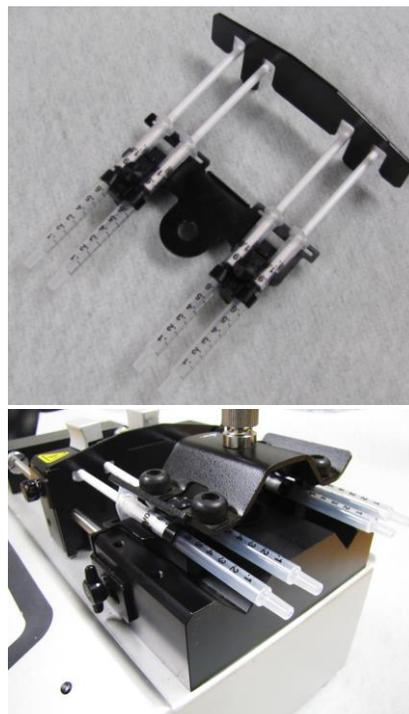
**Figure 5.** Four 1cc syringes secured in syringe rack (top) and secured onto pump (bottom).
