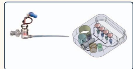
FIGURE 2. Functional decomposition into sample preparation unit and amplification/detection. The four optically clear reaction chambers extend below the cartridge to fit into the fluorometer wells.
