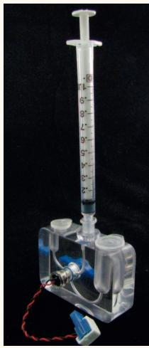
Prototype of integrating the Purelyse® chamber with the Omnivalve™ and two reagent vessels.
